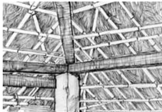
USE OF PRE-CAST CONCRETE COLUMN
