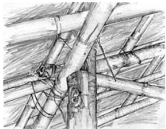
USE OF NYLON ROPES FOR FIXING ROOF STRUCTURES TO COLUMN
