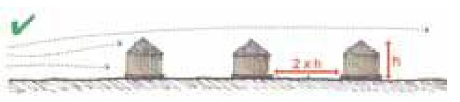
Allow for space between shelters or rows / blocks of shelters whilst taking into account the direction of any prevailing wind
