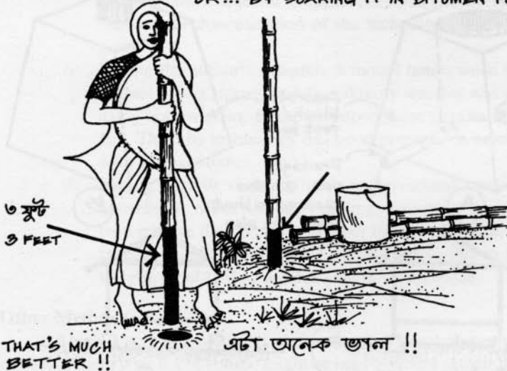
Figure 7: Inexpensive treatment method for bamboo post base (Ahmed, 1994, adapted from Chisholm 1979)
